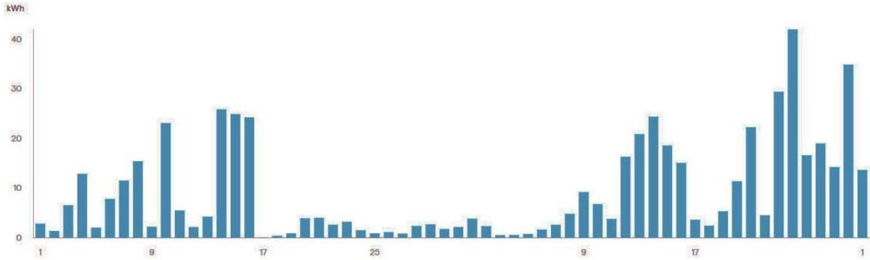
The system generates power throughout the winter but obviously much less than during summer time. On Jan. 17, 2022 there was zero-kWh generated when we had the massive snowfall in less than five hours. It took three days before the system started to deliver power again since most of the panels were covered in snow and ice. It took more than three weeks for the panels to start generating meaningful power with a peak on Feb. 24/22
